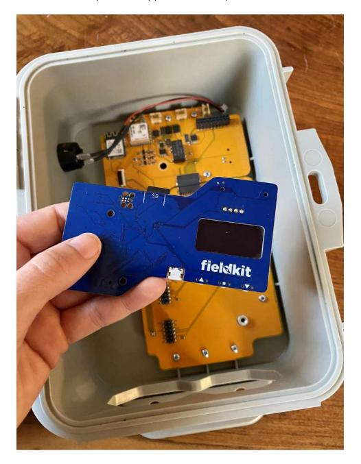
Now it's time to replace the Upper Board on top of the Lower Board.\_\_\_\_\_
