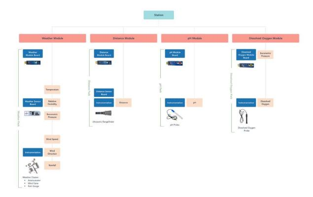
Diagram of a Station with multiple Modules and Sensors
