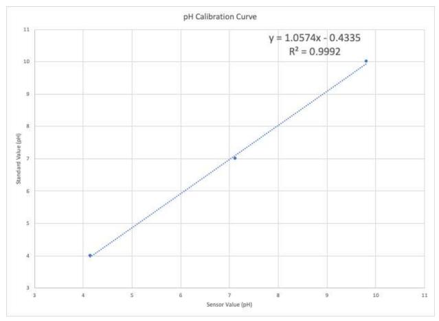
A typical calibration curve, or calibration function, in this case for pH.
