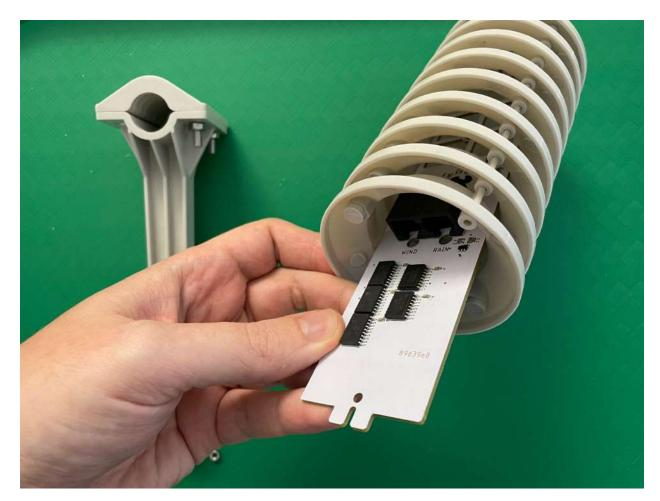
Insert Weather Sensor Board
